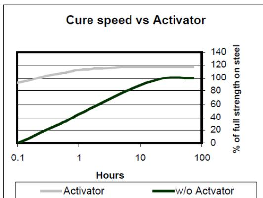
(After 24 hr at 22 °C on degreased 3/8-16 steel Grade 8 nuts and Grade 5 bolts)
