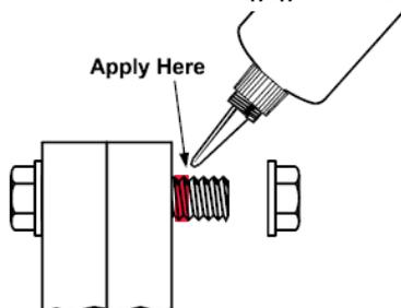
1. For Blind Holes, apply several drops down the female threads into the bottom of the hole. As threads are engaged, compressed air forces the product upwards into the threads.
