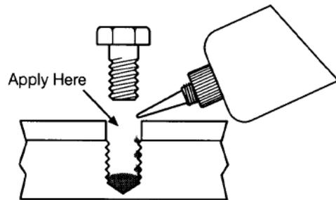
2. Assemble and tighten as usual. When tightening to established torque values, torque compensation is not required.
